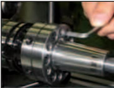
1.4 Position dial gauge at the concentricity check point (ground module collar diameter). Record highest measuring point and “zero” the dial gauge.
